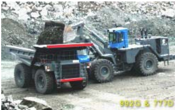
12m 3 -Wheel Loader & 90t-Dump Truck
