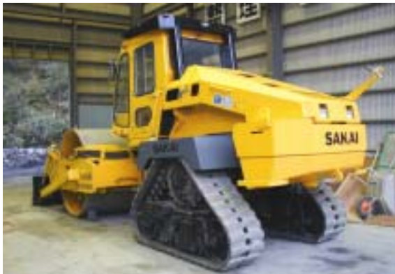
Vivrating roller for Sloop :SV510DVC
