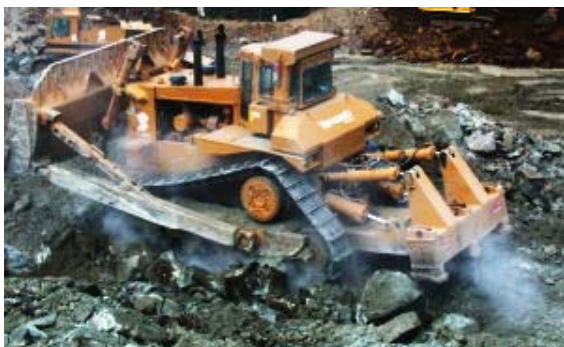
103t-Bulldozer with Ripper : CAT D11R
